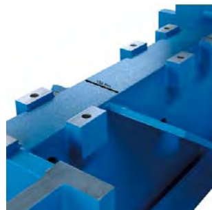
Frame: Main component of the C-frame is 6" thick normalized steel. Elemental analysis designed stiffeners eliminate flex found in cast frames.
