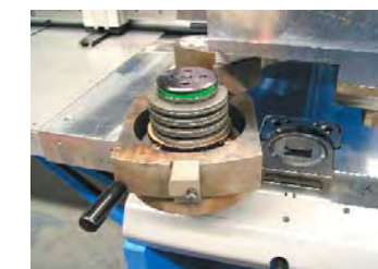
Boschert 4-way and 7-way RevoTool punch heads and die bases. Complete tool sets of customer choice are included.
