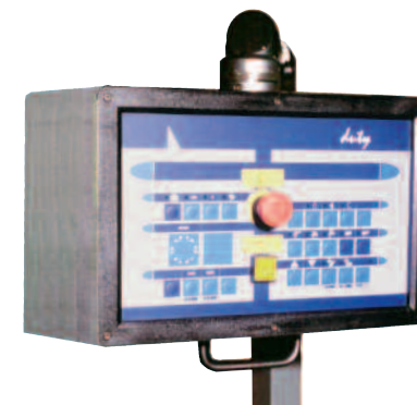
DM-10P Operator Panel Ergonomic design with swing operator control panel allows for easy operation of saw from both sides.
