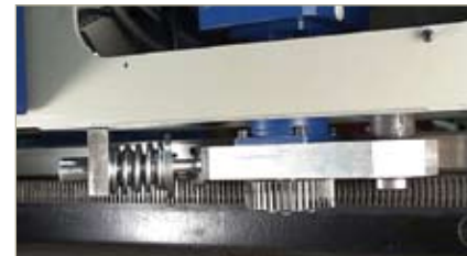
X-Axis Rail and Pinion
