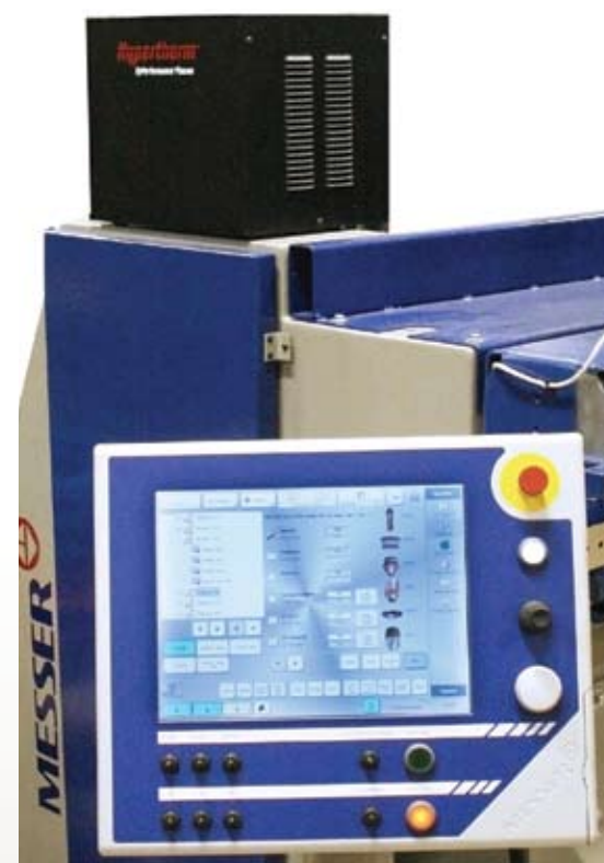
HPR Auto Gas Console with the MG CNC Global Control Plus automates plasma output. No manual adjustments are necessary.
