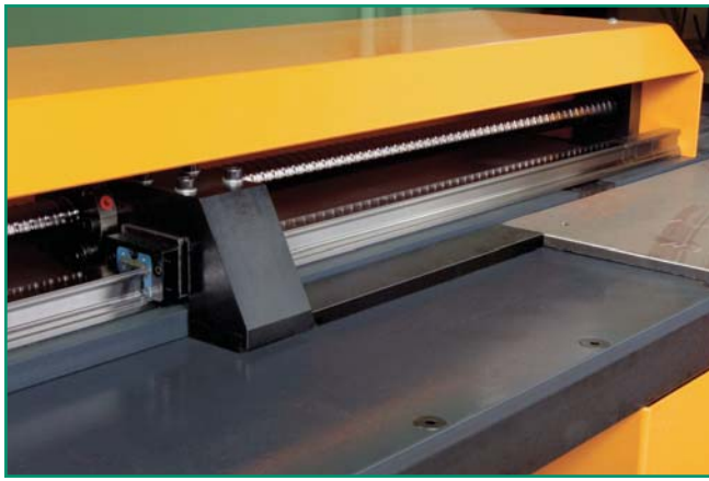
CNC gauging table for X and Y axis positioning.
