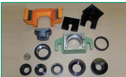
Oversize punch attachment 2-1/2", 3-1/2" (65mm, 90mm)
